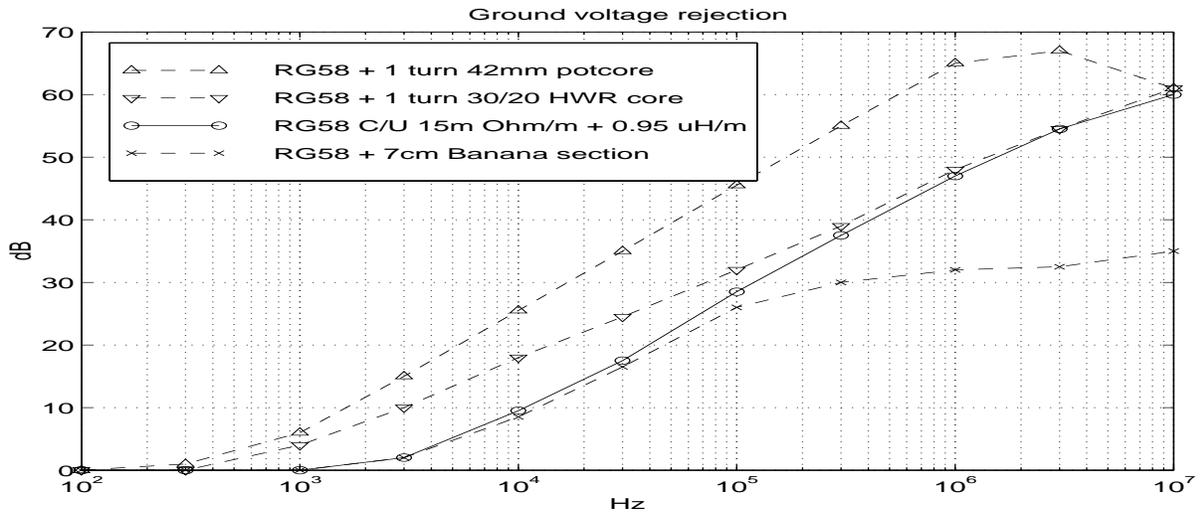
Fig. 4. Ground voltage rejection ( $1/T_v$ ) measurements.
