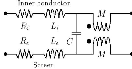
Fig. 2. Co-ax equivalent circuit.
