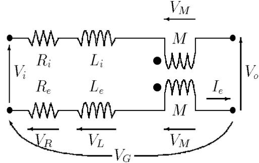
Fig. 3. Ground voltage transfer circuit.
