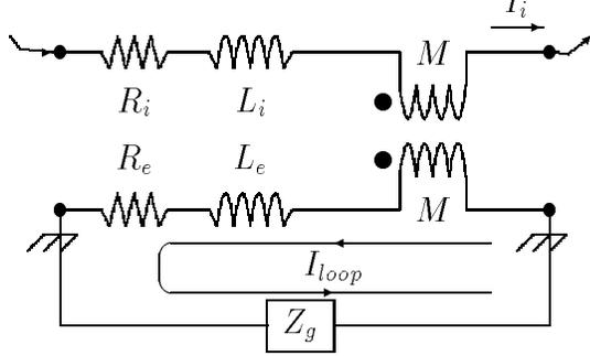
Fig. 5. Induced loop current.
