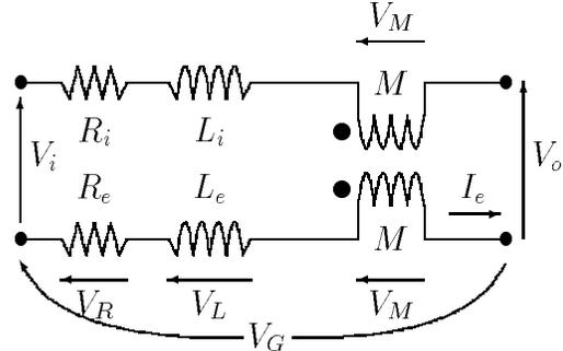
Fig. 3. Ground voltage transfer circuit.
