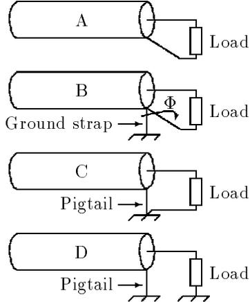
Fig. 8. Four grounding configurations for co-ax at the load end.
