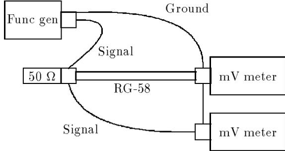
Fig. 9. Test method for ground voltage coupling.
