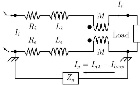
Fig. 7. Ground current = sum of loop and portion of returning signal current.
